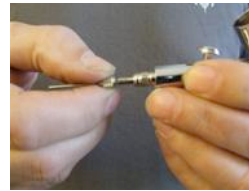
No. 3: Loosen the needle chuck screw 1-2 turn counter-clockwise.
