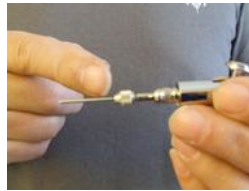
No. 2: This is the needle chuck screw that holds the needle in place.
